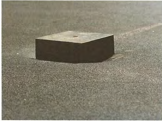
Load Block & Test surface after concentrated loading
