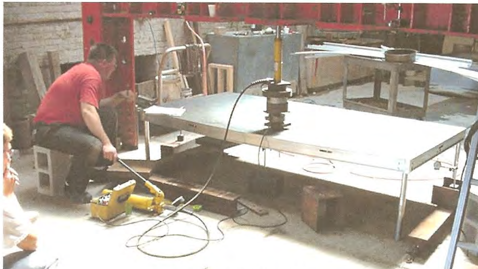
Concentrated load test
