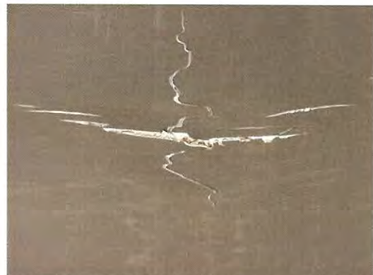
Deformation of lower surface after concentrated loading
