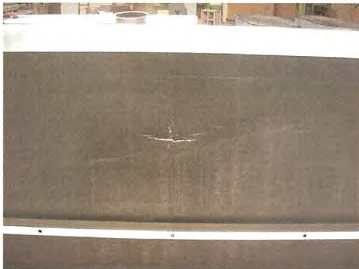
Deformation of lower surface after concentrated loading
